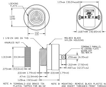
NOTE A: TERMINALS-032 BRASS TIN PLATED, TAPPED FOR #6-32 SCREW. TWO #6-32 NICKEL PLATED BRASS SCREWS INCLUDED. VILL ACCEPT 1/4' QUICK CONNECT. MDUNTING- REMOVE BLACK PLASTIC NUT AND INSERT THREADED FRONT THREUGH 1.25' HOLE PUNCHED IN PANEL, IF GRIENTATION IS NEEDED, NOTE LOCKING FLATS ON DRAWING, SCREW NUT BACK ON. DO NOT OVERTIGHTEN.
